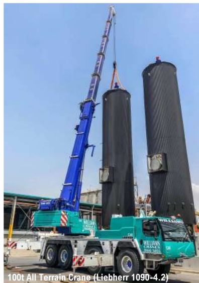
100t All Terrain Crane (Liebherr 1090-4.2)
