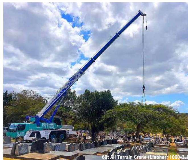
60t All Terrain Crane (Liebherr 1060-3.1)
